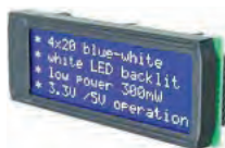
Alphanumeric LCD Modules 4x20 characters DIP204B4NLW is blue with white backlight, other models are with yellow-green LED backlight.
