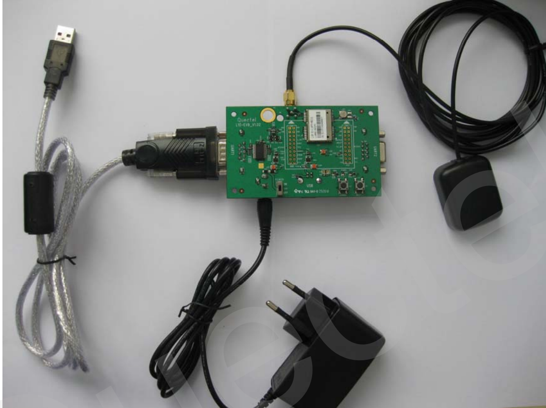
Figure 12: EVB and accessory equipments with serial cable
