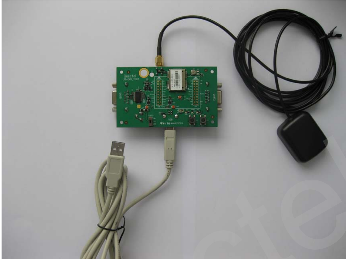
Figure 13: EVB and accessory equipments with USB cable
